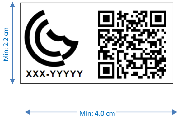
Fig. 2: Minimum dimensions of the GCTS for Certificates
