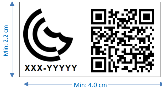
Fig. 2: Minimum dimensions of the GCTS for Certificates
